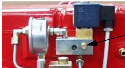
Fig. 15 - Light oil manifold (PG60)
