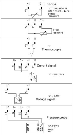
Fig. 25 - Probes connection scheme for modulating burners
