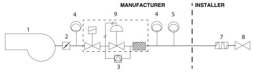
Rp2 - DN65 - DN80: Gas train with valves group VGD with built-in gas pressure governor + gas proving system VPS504
