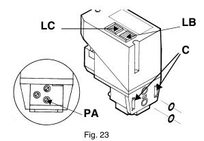
When wishing to monitor the test, install a pressure gauge ranged to that of the pressure supply point **PA** (Fig. 23). If the test cycle is satisfactory, after a few seconds the consent light **LC** (yellow) comes on. In the opposite case the lockout light **LB** (red) comes on. To restart it is necessary to reset the appliance by pressing the illuminated pushbutton **LB**.
