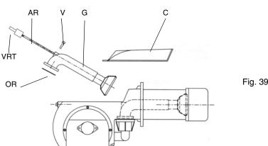
To remove the combustion head, pull it out. Once removed, check that the air and gas holes are not obstructed. Clean the combustion head by means of compressed air or scrape off the scale using a metallic brush.
