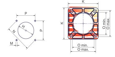
Boiler recommended drilling template and burner flange
